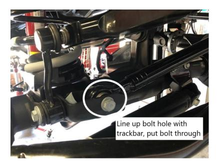
While on ground under Jeeps own weight at ride height, torque all control arm bolts, uppers, lowers at frame and axle. Torque all shock bolts at frame and axle. Torque front trackbar bolt. Check and torque all other bolts. Use chart below for supplied hardware. Use factory specifications for factory hardware.
