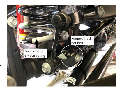
7. After removing all parts specified in the above steps, the lower control arms might bind when lowering the axle. If you remove the axle side control arm bolts, do so **one side at a time**.
