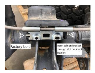
Note: Carefully move line. Do not crimp/pinch line. Always check for leaking fluids and that brakes work correctly. Bleeding brakes is extremely important to be done properly. Follow factory specifications in doing so. Consultation/should be performed by a trained professional mechanic.
