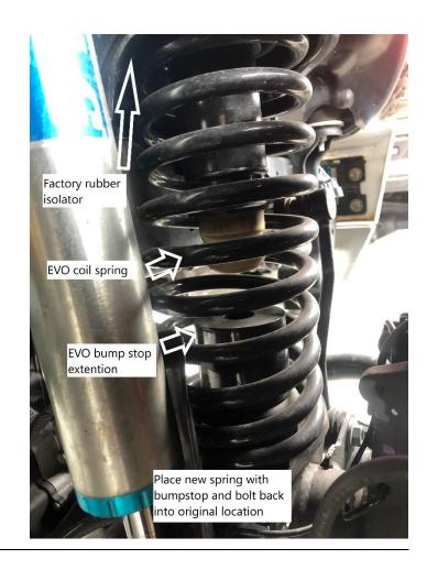
Note: Make sure factory coil seats stay in the factory locations, Left coil seat on the left and right on the right, etc. Also make sure that the rubber pins insert into holes on coil brackets.
