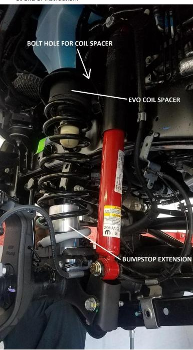
15. Insert supplied 3/8 x 2" bolt into front bumpstop extension. Place bumpstop with bolt inside (bore side up) factory spring and reinstall factory coil spring and rubber isolator on top of coil into its original location on both the frame and axle. Isolator will now be seated on the EVO coil spacer. Axle may need to be lowered to install.
