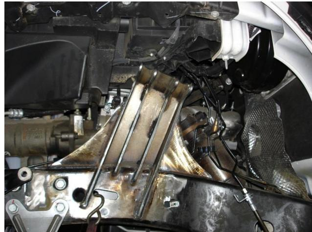
18. Install coilover without springs and bypass shock into upper DTD tower. Coilover should be in front of the vehicle, bypass should be in the rear.
