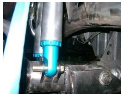
23. Once both shocks on both sides are compressed tack weld lower axle mount to axle tube.
