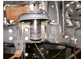
10. Sand frame smooth where coil/shock towers once were and remove paint from surfaces to be welded
