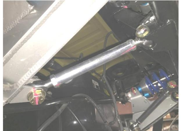
42. Install factory trackbar into frame side mount in factory orientation with factory hardware
