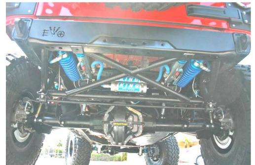
45. Install Coilover into EVO arm on driver side with spacers and 1/2" x 2.5" hardware. Repeat these steps with Bypass shock.
