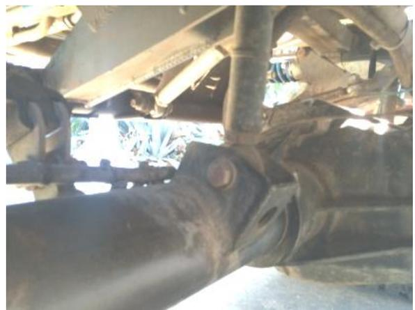
40. Assemble EVO cross brace links, thread jamb nuts on each heim and thread each heim into cross brace tube.
