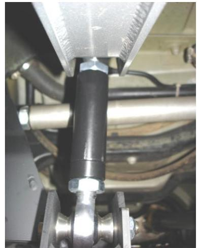
37. Using  $\frac{1}{2}$ " hardware install opposite end of EVO endlink into driver side axle trackbar mount
