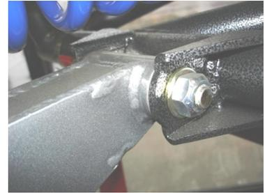
21. Place axle trackbar bracket into place on axle pad
