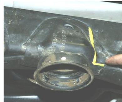
26. Install Frameside Trackbar/bumpstop bracket into place. Install 1/2" x 1" bolt from factory trackbar bracket through into EVO bracket
