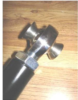
36. Using  $\frac{1}{2}$ " hardware install one end of EVO endlink with mis-alignments into large end of EVO arm on driver side
