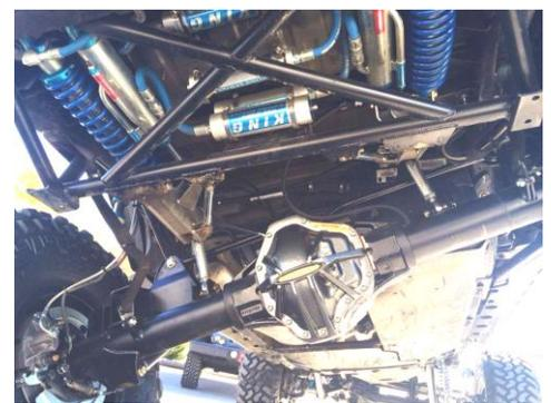
46. Install Coilover into rear mounting location on passenger side with spacers and 1/2" x 2.5" hardware. Repeat these steps with Bypass shock.
