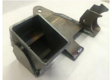
25. Grind bumpstop mount on frame smooth as seen in photo. Passenger side only.
