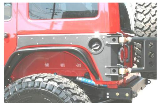
48. Coilover Reservoir tabs can either be mounted on the outside of the frame or on the EVO subframe with Bypass Reservoirs. Use two tabs and two hose clamps per reservoir.
