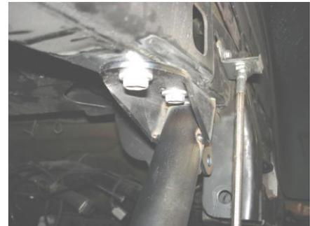
20. Install assembled EVO arms to pivot locations on the subframe with supplied 9/16" hardware
